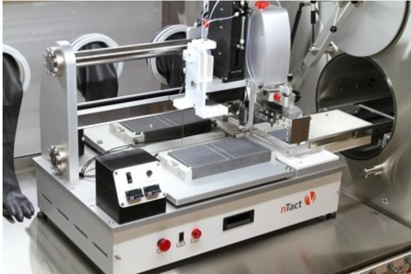
*The M Braun Group and nTact will jointly offer a glove-box and a slot die coater in one complete system*
